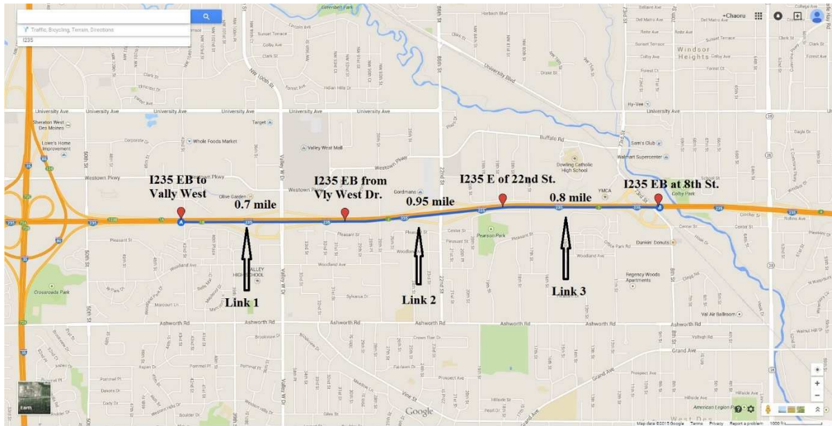
Figure 3.6 Study Corridor and Sensor Locations (source: ©2015 Google)
